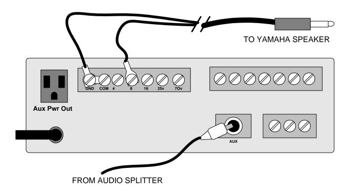
Notes: Aux Pwr Out is used to feed the tape deck it's power.
